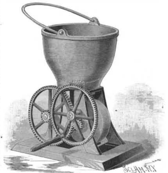
CLEGG'S PLUMBER'S FURNACE.
