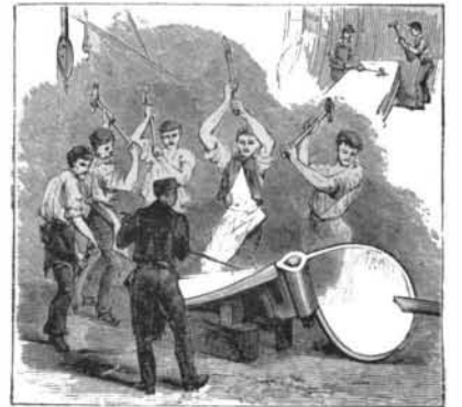
FORGING STEEL SCREW PROPELLER.
