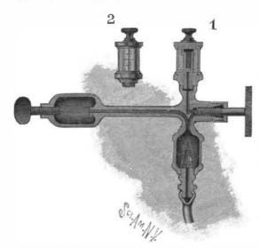
MIXING AND VAPORIZING DEVICE FOR INHALERS.
