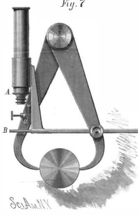
Now, it must be admitted that the portion of the tool that really does the work is microscopic in its dimensions, and a comparison of two such tools by the aid of a microscope will reveal the cause of inferior work with one tool, and the reason of good work with the other tool. The character of the cutting edge depends altogether upon the temper of the tool and the means and methods employed for sharpening it. A tool ground upon a coarse emery wheel or grindstone will
