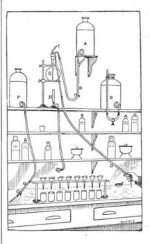
one of the holes issues a rubber tube, D (or glass with rubber connections), descending to the desk and ending in a glass nozzle. Connection is made by a second hole in the stopper with a reservoir botabove the top of the washbottle. In the third hole is placed a glass tube bent at an angle to keep out dust. On filling the flask from the reservoir-the flow being stopped
