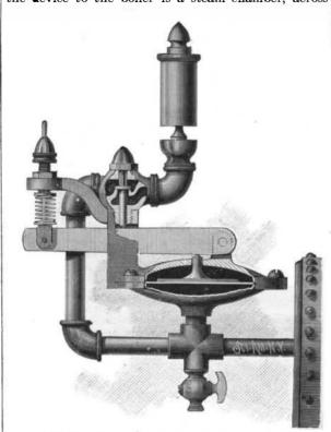
SAFETY VALVE AND ALARM FOR STEAM BOILERS.
