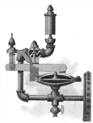
SAFETY VALVE AND ALARM FOR STEAM BOILERS.
