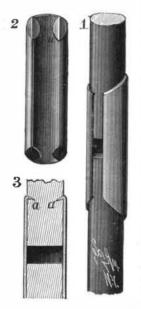
against the closed side of the clip. It will be seen that both ends are so secured that any strain put on the belt will only tend to force the ends of the belt further up the inclined projections. There will be no tendency the bath long enough to become chilled. The traof the belt ends to come out of the open side of the elip, and the strain will not tend to force the sides of the clip apart.
