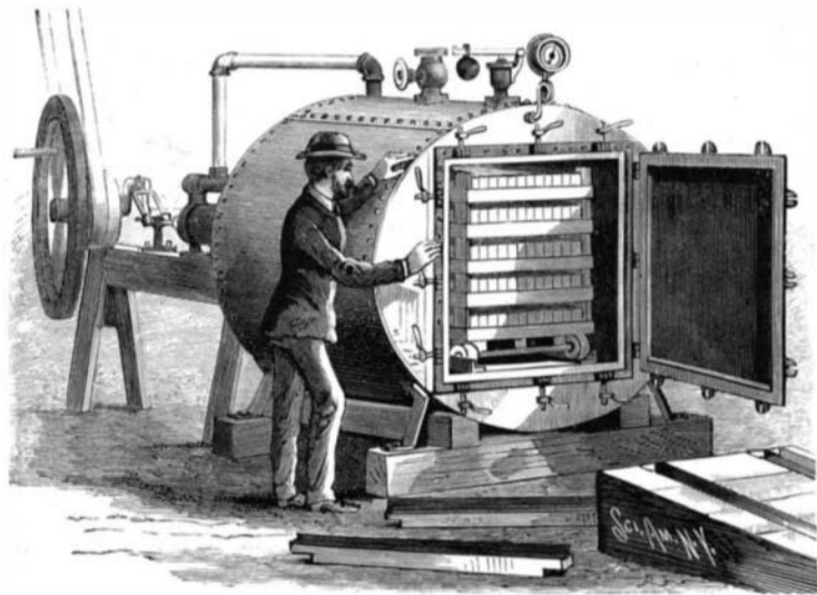
HUTCHINGS' APPARATUS FOR TESTING SEALED CANS.
