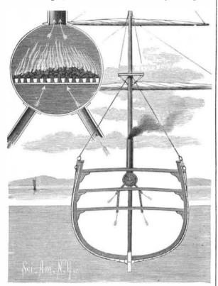
BARTON'S NEW SYSTEM OF VENTILATING VESSELS.
