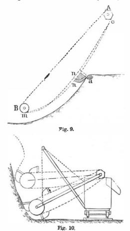
to attack a greater height (as is done in practice), we proceed to undermine the earth (Fig. 10), the jfb becomes involved in the latter, and the apparatus comes to a standstill. The apparatus of the second category have the same drawbacks, but are nevertheless superior as regards their power of work ing in a forward direction.
