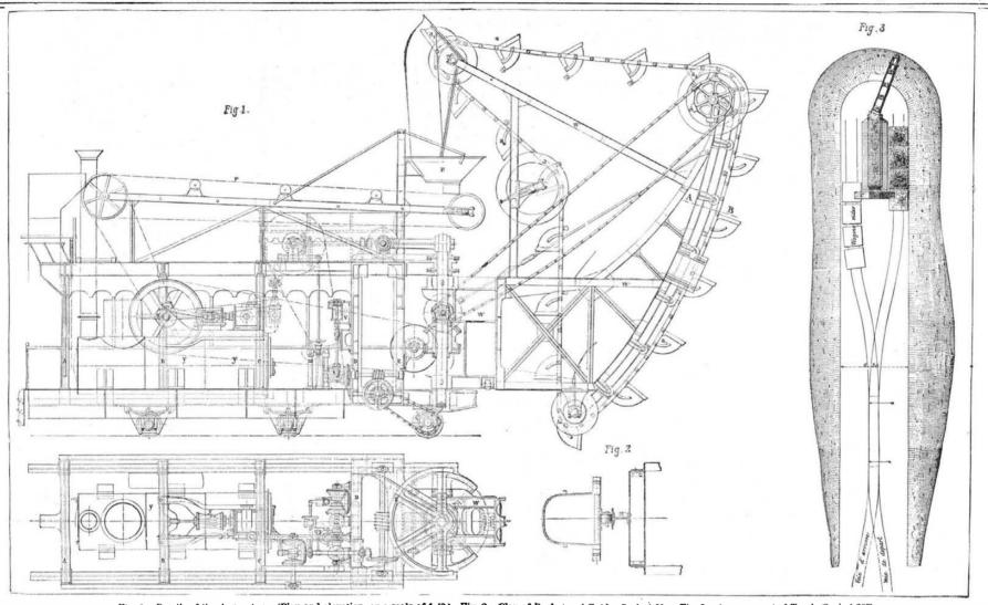
Fig. 1.—Details of the Apparatus. (Plan and elevation, on a scale of 1-40.) Fig. 2.—Plan of Bucket and Guide (Scale 1-20). Fig. 3.—Arrangement of Track (Scale 1-200)
