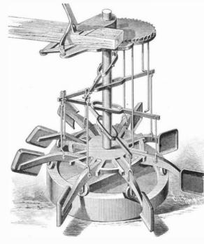
the lever is moved toward the disk, the brakes are moved out of contact with the disk, which is made to revolve backward by the pawl engaging against one of the teeth. The disk is connected with the shaft by a spring catch, and is thereby adapted to revolve with the wheel.
