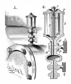
HORN'S ENGINE LUBRICATOR.
