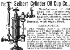
Manufacturers of Oil Cups for Locomotive, Marine and Stationary Engine Cylinders, under the Seibert and Gates Patents, with Sight Feed.
