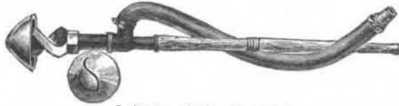
BOILER FLUE CLEANER.
