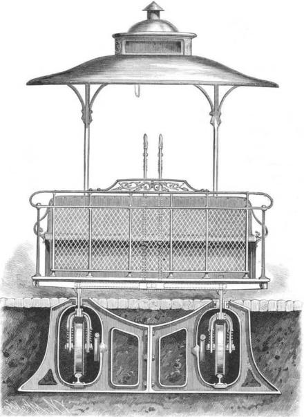
two slots appear which communicate with two tunnels, constructed in the following manner:
