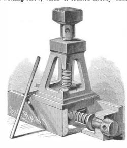
QVARNSTROM'S IMPROVED LIFTING JACK.
