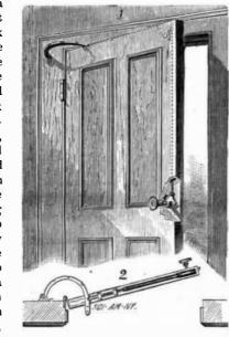
as it passes the center, so that it will hold the bolt in an unlocked position. By means of this simple contrivance the door may be locked at any desired angle, or the bolt may be secured in a withdrawn position, so that the door may be opened or closed as if no check had been applied. Fig. 2 is a view of the top of the door. This invention has been patented by Mr. Thomas B. McCurdy, of Lancaster, Texas.
