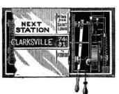
be sounded to call the attention of the passengers to the station indicator. The rollers ar provided with clutching devices whereby the loose cogwheel (with which each roller is provided) of either roller can be engaged with a cogwheel operated by the clockwork mechanism, whereby the band can be wound in one direction or the other, according to the direction of the train. This invention has been patented by Mr. John W. Watts, of Clarkesville, Mo.
