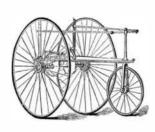
the axles through the ratchets and pawls, instead of cranks, as commonly arranged. By this means dead centers are avoided, and the wheels may continue to run when the treadles have ceased to act, allowing the operator to stand on them without working the machine, thus
