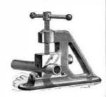
ing double inclines and being held loosely in the frame of the vise, it will be seen that when the turning power is apinclines to grasp the pipe with increasing firmness, accordno danger of the pipe slipping or turning between the been patented by Mr. Alfred Beard, of Danville, Ill., who may be addressed for further information.
