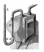
preventing the escape of gas following the destruction of the meter or the melting of the connection. Our suggestion has been heeded by Mr. Fred R. Hoard, of Providence, R. I., who has invented the simple and effective device shown in the engraving. It consists of a hollow ball, B, filled with lead or fusible metal with the exception of a central passage. This ball is inserted in the
