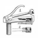
receiving the body of the cartridge shell, and the handle has an anvil above the center of the apertured portion of the main arm, so that when a shell is passed through the aperture with its flange resting upon the upper side of the arm, the primer or cap can be forced into the shell by means of the handle and its anvil as shown in Fig. 1. Upon
