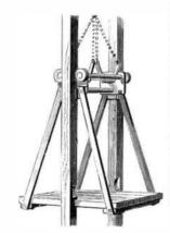
car is being supported by the ropes or chains the cams are held out of contact with the uprights, but when the ropes give out a spring connecting two arms of the shafts brings the cams into engagement with the uprights and arrests the car. This is very simple in its construction, easily applied, and certain in its operation.
