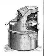
upon by the animal as he sinks downward with the swinging platform, in order that he may not be startled and turn back until it is too late for him to get out. The trap is provided with a catch bolt, which may be made to hold the platform until the trapper desires to trip it by means of a cord attached to the bolt. This novel and effective trap has been patented by Mr. T. B. Turley, of La Mine, Mo.
