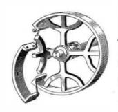
and taken off without unlacing it, and maybe readily slackened at any time for any purpose. In smaller sizes of pulleys the inventor proposes to cast the removable or adjustable portion of the arm and its branches, when used together. with the removable section, and connect it with the fixed part.
