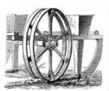
crusts with hoes to enable the corn sprouts to come up. The wheel has two narrow tires of in mounted on branch spokes, the tires being placed a little distance apart, and having the inner edges turned inward or toward the hub to leave a narrow ridge of softearth with sloping sides that will shed the rain well This invention has been patented by Mr. J. McDaniel, of New Hampshire, O.
