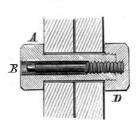
is to screw for drawing up the bolt on the plates. The nut has another and smaller socket or bore, threaded to receive the end of a binding screw, which is screwed in from the head of the bolt by a wrench or screw driver, after nut is screwed on. For long bolts the socket in the
