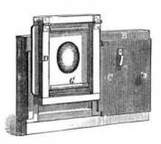
grooved tracks, B, are attached to the printing frame, and in these tracks a slide moves, one half of which is open, and over this open part a sliding box frame, D, isheld by guide strips in such a manner that the box frame may move transversely over the slide. The
