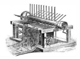
carpet to be whipped is placed, is composed of a series of rods placed in a rectangular frame, this frame being pivoted to the main frame. The outer edge of the table is supported apon a board that is adapted to be moved rapidly up and down by a rack and pinion. The rapid vertical vibration of the carpet, with the beating, causes the dirt to be rapidly and thoroughly removed from the carpet.
