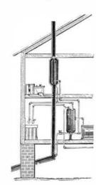
heat the air in the soil pipe, causing a draught which carries off all the foul gases through the pipe and out at the roof. As the water cools it sinks to the bottom of the vessel and is carried back to the heater, and in this manner a continual circulation is maintained in the vessel, and consequently continual draught through the soil pipe is secured.
