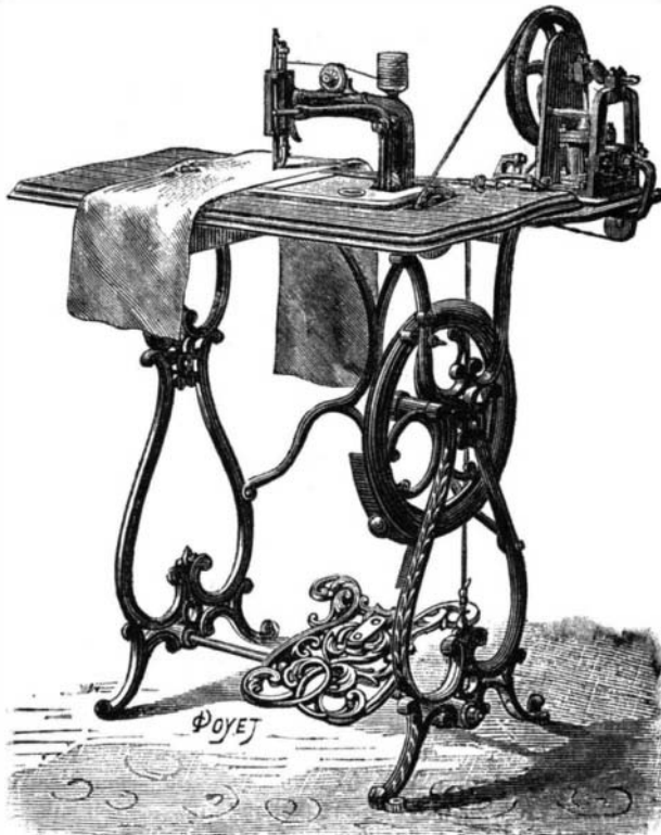
Fig. 2.—RAREFIED AIR MOTOR APPLIED TO A SEWING MACHINE.
