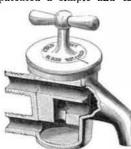
hot or cold water may be drawn separately, or both may be drawn at the same time. The barrel of the faucet is made tapering, to form a seat for the plug, which is held in the ordinary way. The plug has the usual handle, and has also a dial on the plug for indicating the character of the water discharged, that is, hot, cold,
