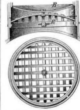
Inside of the smokestack is placed a concavo-convex grate, formed of parallel bars attached at their ends to a rim. This grate fits into the upper part of an outer rim, C, and has guide pins which enter vertical slots in the rim. The rim, C, is fitted into the smokestack, and rests
