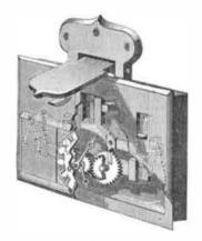
graving. The lock casing is provided on its fron' side with a recess, in which is placed a dial, and also upon the case are two beveled ridges in which a plate slides for covering the face of
