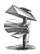
be raised to an upright position, exposing the fruit upon the scaffold to the full rays of the sun, and may also be turned to a vertical position. The fruit is protected from rain or dew by swinging the shelves together and lowering the roof over them. This invention is patented by William Smith Haley, of Columbia, Tenn.
