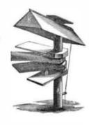
be raised to an upright position, exposing the fruit upon the scaffold to the full rays of the sun, and may also be turned to a vertical position. The fruit is protected from rain or dew by swinging the shelves together and lowering the roof over them. This invention is patented by William Smith Haley, of Columbia, Tenn.
