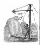
serted in the hay, and draught applied to the lifting rope, which elevates the fork and runs it forward, when it is tripped to unload. When the apparatus is not required for use, it may be packed away in close compass. This hay stacker has been patented by Mr. James Wilson, of Marengo, Iowa.
