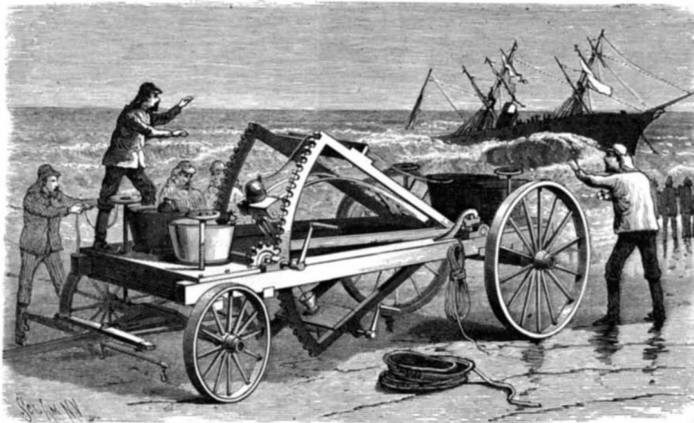
CLAYPOOL'S CATAPULT FOR THROWING LIFE LINES
