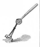
them together to grip any object placed between them. By removing the key the parts can be so placed in relation to each other that the clamping device shall be at any desired angle with the handle, and they are secured in this position by replacing the key.
