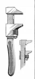
adjust it to its work, so that only a slight turn of the screw is afterward necessary to give the requisite grip. The same construction also provides for the rapid removal of the serrated jaw from the bar and over and off the skeleton handle. When the wrench is in use the harder the strain thrown upon the jaw the firmer will the screw engage with the rack. The tool can be very quickly changed from a nut wrench to a pipe wrench.
