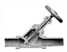
manner. When the valve is opened a nearly straight, unobstructed passage is provided for the fluid, and the friction of the flow of the fluid is reduced to a minimum. In the check valve the stem has a longitudinal aperture opening at its side into the outlet portion of the valve chamber, thereby prevacuum action.
