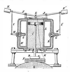
have at their outer end weights, K K'; at their inner ends they engage with a latch, L, at the center of the cylinder. Steam or water is admitted through the pipes, GE, to the cylinder, and the block is pressed down until it is sufficiently cut away, when the latch is released by a chain, M, connected with the presser, D, when the weights fall, reversing the cocks and raising the piston and presser block.
