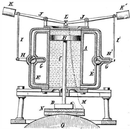
have at their outer end weights, K K'; at their inner ends they engage with a latch, L, at the center of the cylinder. Steam or water is admitted through the pipes, G E, to the cylinder, and the block is pressed down until it is sufficiently cut away, when the latch is released by a chain, M, connected with the presser, D, when the weights fall, reversing the cocks and raising the piston and presser block.
