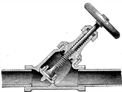
manner. When the valve is opened a nearly straight, unobstructed passage is provided for the fluid, and the friction of the flow of the fluid is reduced to a minimum. In the check valve the stem has a longitudinal aperture opening at its side into the outlet portion of the valve chamber, thereby preventing any retardation in the movement of the valve by vacuum action.
