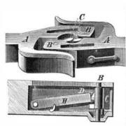
with their ends against the bottom of the spiral shoulder, D, and prevent the hooks, C, from swinging outward. In coupling the hooks, C, will face each other, and swing inward sufficiently to allow the shanks of the drawhead to pass into each other, when they swing out and the cars are coupled. When the latch, H, is raised and the cars drawn apart, the hooks, C, turn each other outward and the cars separate.
