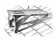
that pass through longitudinal slots in the top, thereby adapting the seat to roofs of different inclinations To adapt the braces. C, to this adjustment of the top they are rigidly secured to the sides of the support, B, but are adjustably attached to the top, A,
