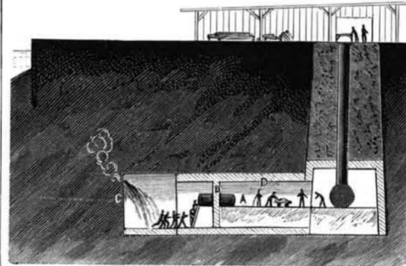
Fig. 1.—SECTION OF THE TUNNEL, CAISSON, ETC.
