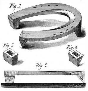
used in connection with this shoe. They are held in place by pins passing through both lug and calk.
