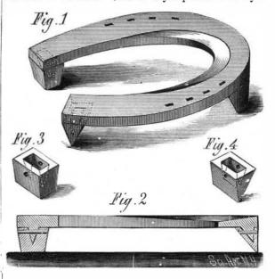
used in connection with this shoe. They are held in place by pins passing through both lug and calk.
