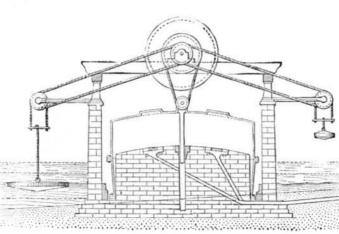
Fig. 1.-Float and Iron Compressing Bell.
