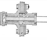
two parts, permits either of them to be removed, to repair the wheel, without disturbing the other, or even removing the wheel from the axle.
