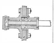
two parts, permits either of them to be removed, to repair the wheel, without disturbing the other, or even removing the wheel from the axle.
