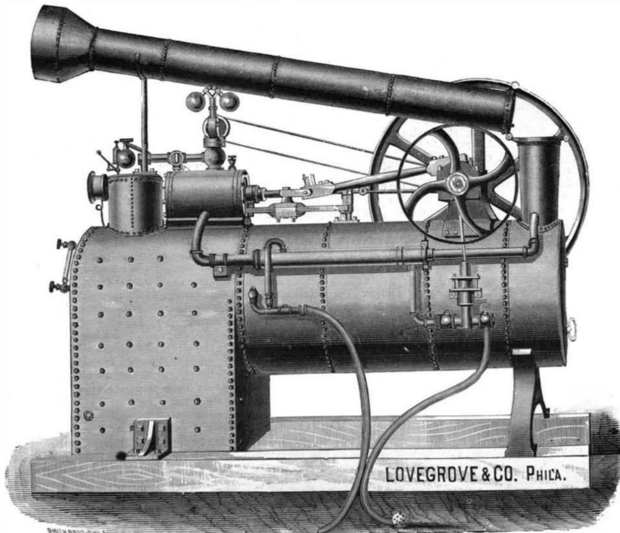
**PHOENIX FOUNDRY AND MACHINE CO.'S PORTABLE ENGINE.****Civil Engineers.**
