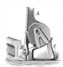
contiguous rails, where great difficulty is experienced in applying an ordinary claw-bar, by resting the lower edge of the eccentric on the top of the rail; with the bar, A, inclined slightly rearward, the claw may easily grasp the spike, and by motion of the lever drawn, the swinging fulcrum resting unused on the outside of the rail.
