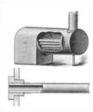
remove a flue a skilled workman must be employed. By this construction it will be seen that the flues are detachable and can be inserted or removed by an ordinary workman, and they serve also as braces to the flue sheets. The inventor claims that by the employment of copper nuts a galvanic action is created between the copper nuts and the iron threads on the ends of the flue which prevents the iron threads from rusting, whereby their strength is impaired, and the copper nuts will not oxidize.
