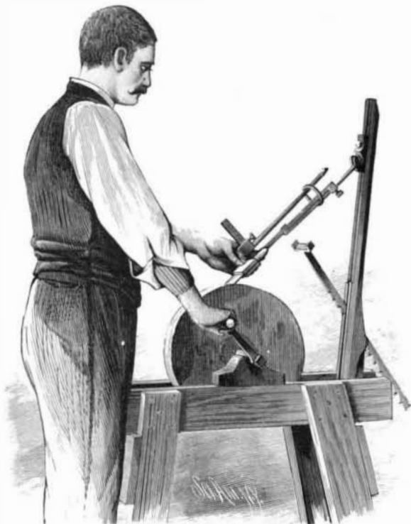
BAYHA'S TOOL HOLDER FOR GRINDSTONES.
