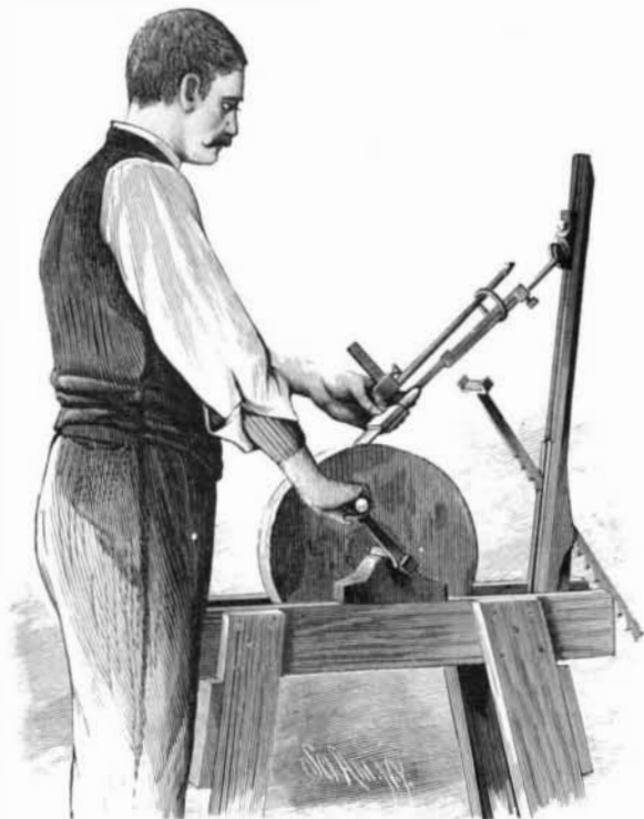
BAYHA'S TOOL HOLDER FOR GRINDSTONES.
